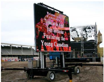
Custom trailers transport 12.5-foot-tall by 16.7-foot-wide LED screens to and from each event at the Calgary Stampede rodeo and entertainment show in Calgary, Canada. Each mobile LED screen consists of 25 Lighthouse Technologies LH 1650D LED panels.
